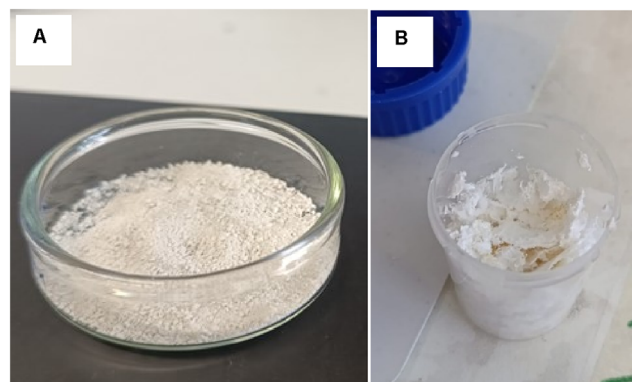
Figure 2. P(3HB) extracted from the biomass produced by B. thailandensis using the hydrolysate as feedstock by applying the enzymatic method (A) and by applying solvent extraction with chloroform (B).
