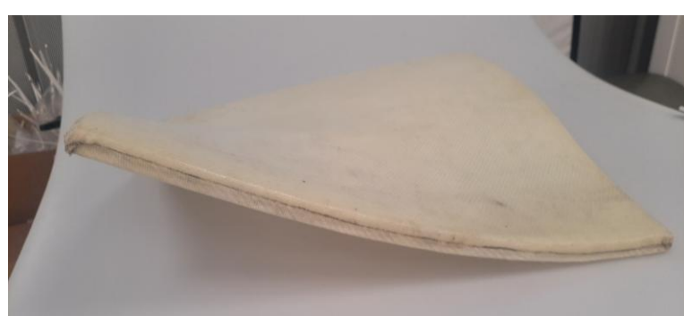
Example of small scale sandwich prototype with double curvature made of FR-LDPE/ glass fibre composite skins and PET structural foam, 500 mm x 500 mm, manufactured by VAT.
