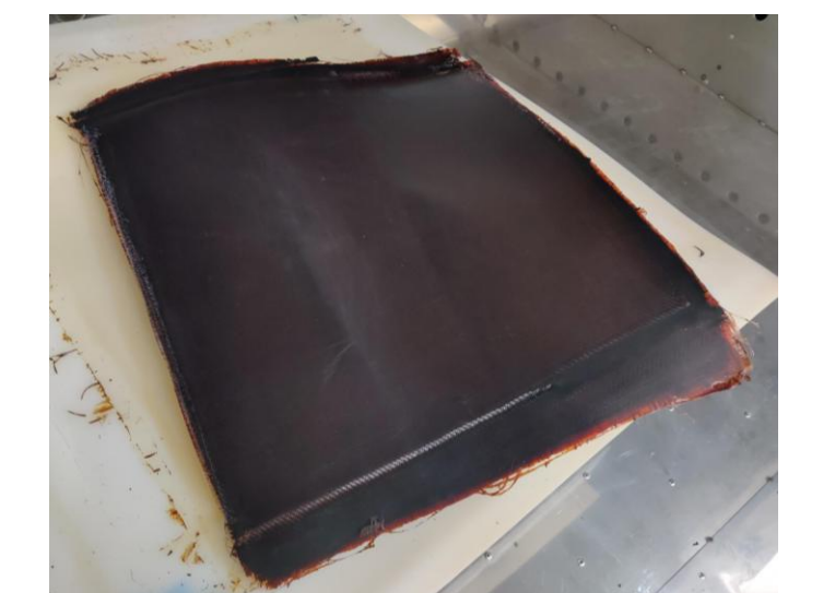
Example of small scale sandwich prototype with double curvature made of furan resin/ glass fibre composite skins and PET structural foam, 500 mm x 500 mm, manufactured by VARI.
