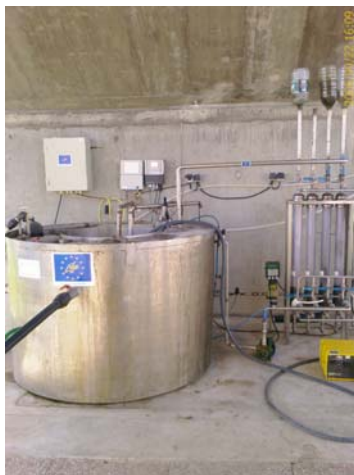
Figure 2. On line monitorization parameters (COD, NO 3 and TSS) in pilot membrane bioreactor (MBR)
