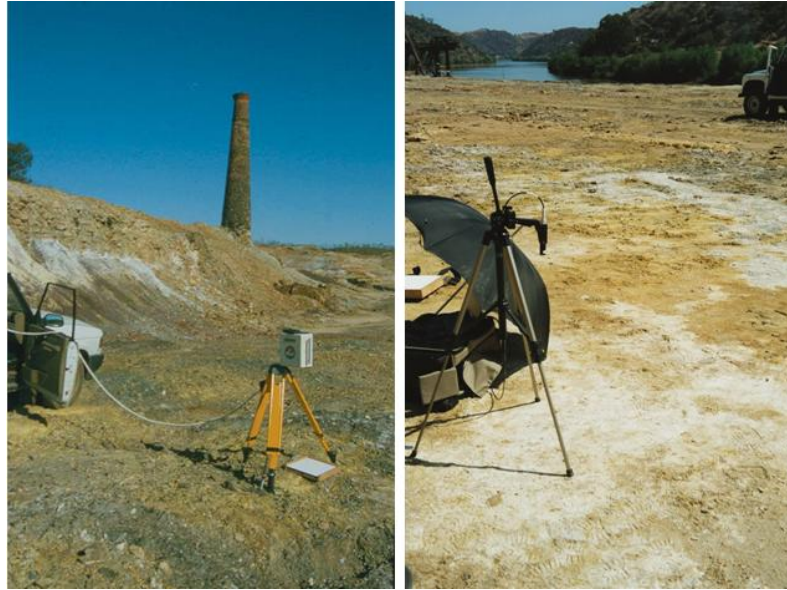
Figure 2. 5 Field measurements with an ASD Fielspec spectrometer (BGR) (Chapter 3). Right-measurements under high temperatures.
