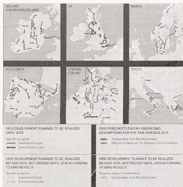
Fig. 13: Summary of EWIS identified network strengthening measures
