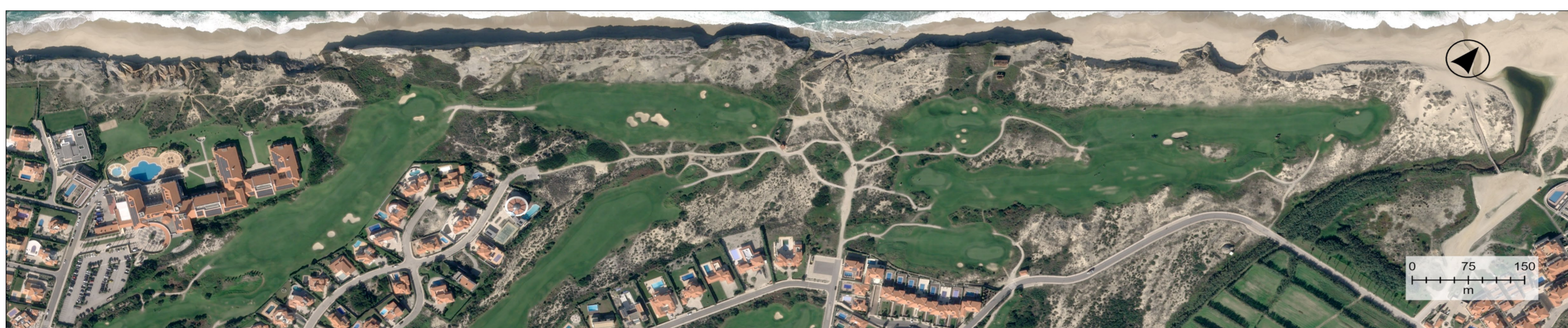
Figure 2 - Pléiades Neo 4 pansharpenerd multispectral ortho composite (30 October 2024; GSD 0.30 m). Standard PMS Full-Scene product, orthorectified by Airbus.
