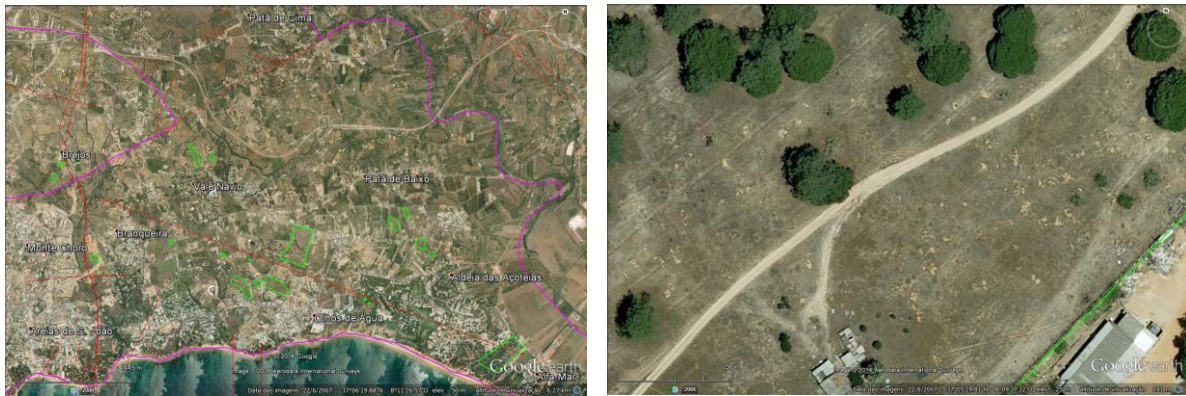
Fig. 2.7 - Overview of the identified subsidence dolines areas (green contour) in the aquifer system (pink contour) (left). Satellite image detail of the depression areas (right). Main faults – red lines. ©Google 2014.
