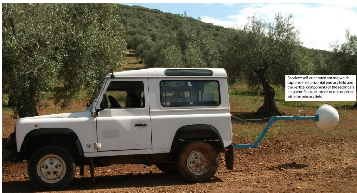
Fig. 2.9 - RF-EM equipment coupled on a vehicle: the receiver antenna is self-orientated and captures the horizontal primary field and the vertical components of the secondary magnetic fields, which are in-phase or out-of-phase with the primary field.
