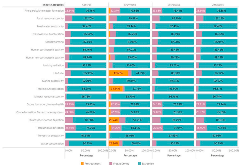
Fig. 9. a) Environmental impacts of the supercritical carbon dioxide extraction of Chlorella vulgaris (Cv) and smooth Chlorella vulgaris (sCv) with pretreatments (bars): enzymatic, microwave, and ultrasound, compared to the untreated biomass (control – dashed line); b) process contribution analysis for steps in microalgae supercritical carbon dioxide extraction with enzymatic, microwave, ultrasound pretreatments, and the untreated biomass (control); c) hotspot analysis of different input categories (infrastructure/equipment, electricity, and chemicals) for microalgae supercritical carbon dioxide extraction with enzymatic, microwave, and ultrasound pretreatments, and the untreated biomass (control); d) Impact reduction of the improvement scenario from baseline for control, enzymatic, microwave and ultrasonic pretreatments.
