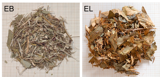
Fig. 1. Macroscopic appearance of the RBE types used in the pyrolysis experiments: (EB) E. globulus branches, (EL) E. globulus leaves.
