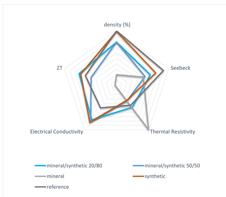
Figure 1 - Radar graph summarizing the TE properties of some representative START samples, measured at 350 °C. To help visualization, each axis goes from zero or from the value of minimum acceptability to the maximum value measured for each property, for this class of materials. Density (%) is the density of the sintered pellet with respect to the density of the powder material. Axes spans: (density (%): 80-100; Seebeck: 100- 250 ( \mu\text{V}\cdot\text{K}^{-1} ); Thermal resistivity: 0.5-3 ( \text{m}\cdot\text{K}\cdot\text{W}^{-1} ); Electrical conductivity: 0-20 ( \text{mS}\cdot\text{m}^{-1} ); ZT: 0-1. In general, a bigger area identifies a better performing TE material.
