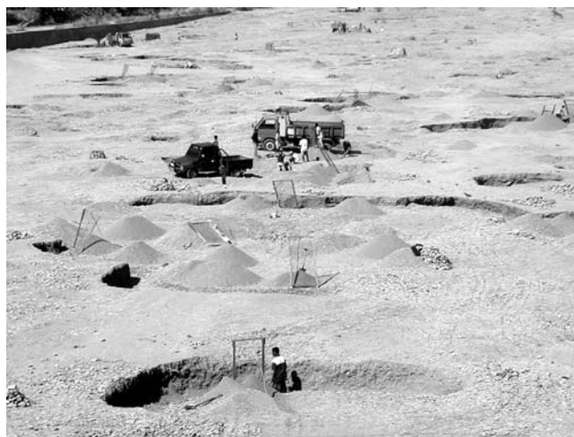
Fig. 19. Sand and gravel exploitation in Comoro River, Dili. Note the numerous small pits dug by local miners.
