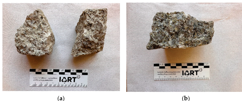
Figure 1. (a) Greisenized granite (zinnwaldite mica-poor GCW-1; (b) greisen (zinnwaldite mica-rich GCG-1).
