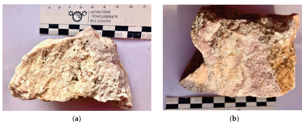
Figure 2. Lepidolite-bearing aplite (LSA-1, (a)) and feldspar-lepidolite pegmatite (LSR-1, (b)).
