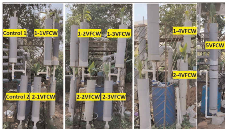
Figure 2 | Pilot-scale demonstrated 2-stage vertical flow constructed wetland types.
