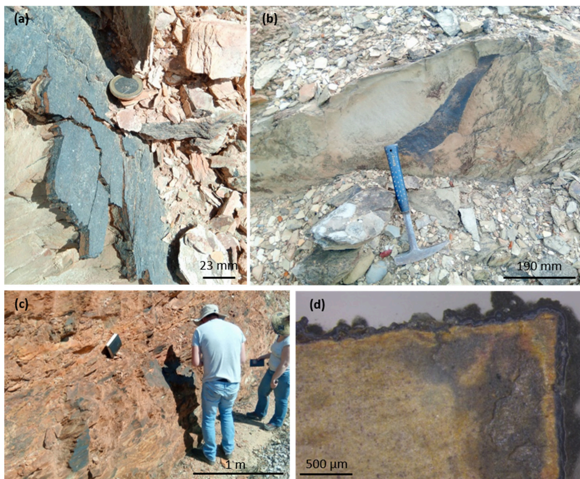
Figure 3. Examples of rock coatings collected on the Neves-Corvo mine area rock outcrops. Black colors represent zones enriched in iron (Fe) and manganese (Mn). (a) Rock Fe-Mn coating in the diacalse zone of Grandaços Fm. (Volcano–Sedimentary Complex). (b) Rock Fe-Mn coating in the greywacke cleavage (Mértola Fm.). (c) Fe-Mn outcropping-rich zones of the Grandaços Formation shales. (d) Rock coating cross-section (Grandaços Formation shale).
