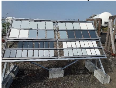
Fig. 3. Samples exposed at the testing site with category C5 (for steel) environmental corrosivity.
