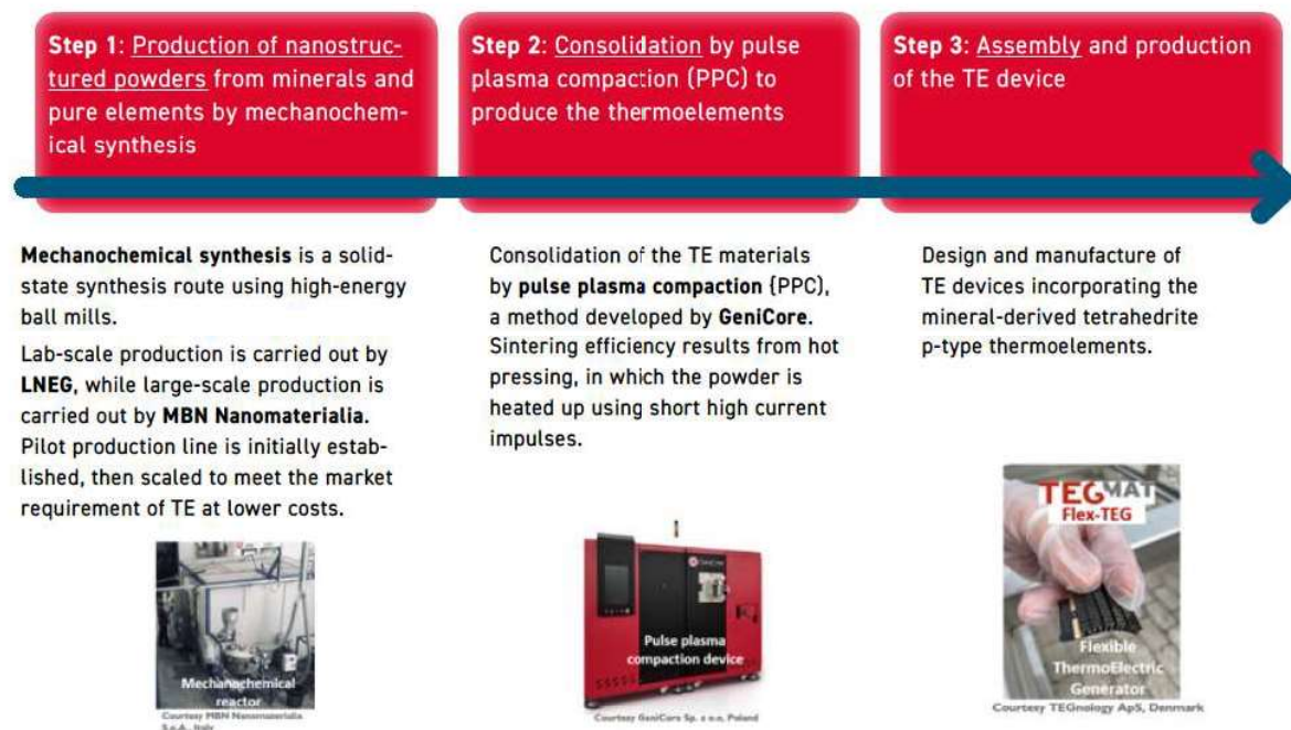
Fig. 4 The START process workflow. The main partners involved in these activities are nanostructured powder specialist MBN Nanomaterialia, for Step 1; material engineering company GeniCore, Step 2; and TEGnology, a leading company in TE energy harvesting, Step 3.
