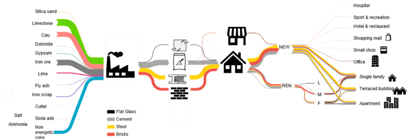
Fig. 5. Annual average material flows for building construction and renovation in the overall EU+. New stand for new construction and REN stand for renovation. L stands for light renovation, M for medium renovation and F stands for Deep renovation. Common sand is not represented.
