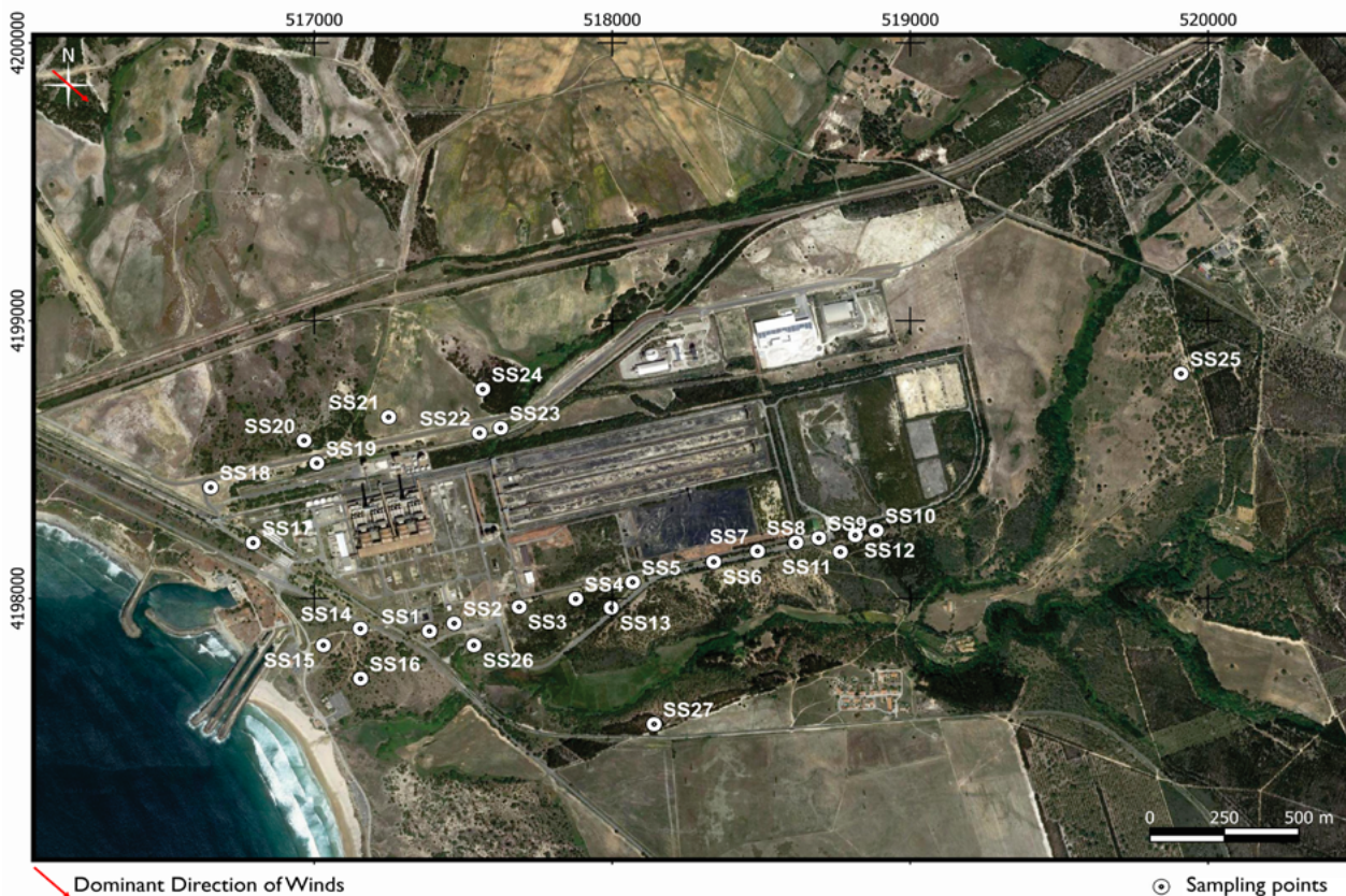
Figure 2. Aerial image of the STPP with identification of sampling locations and dominant direction of winds.
