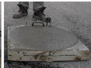
The diameter of the resulting flow is measured
