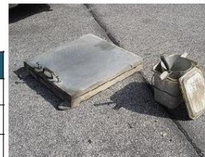
Equipment; flow table, Abrams cone, waterbucket and broom.
