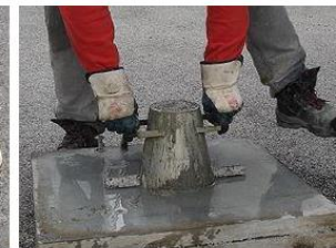
The cone filled with concrete, prior to lifting.
