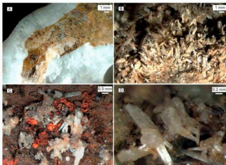
Figure 9. Stereomicroscope images of aragonite (A) from third level (sample PR53); (B) mine waste open pit (PR66–fragment 12); and cerussite from mine waste open pit: (C) sample PR66–fragment 3; (D) detail of sample PR66–fragment 6.
