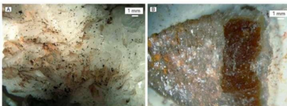
Figure 10. Stereomicroscope images of: (A) dolomite+minrecordite from third level (sample PR9); (B) calcite+ankerite (PR27).
